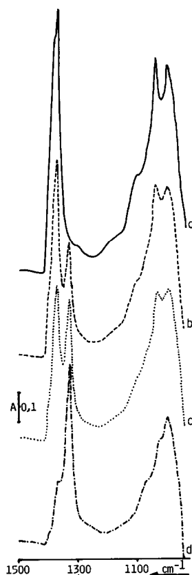
FIG. 5. Spectra of sulfated \text{TiO}_2 during exchange with \text{H}_2^{18}\text{O} at 450^\circ\text{C} . (a) Sulfated sample after oxidation of 200 \mu\text{mol g}^{-1} of \text{SO}_2 . (b) After 1 h exchange in 2.5 Torr of \text{H}_2^{18}\text{O} then evacuation for 30 min at 450^\circ\text{C} . (c) An additional 1 h exchange in 5 Torr \text{H}_2^{18}\text{O} . (d) An additional 1 h exchange in 12 Torr \text{H}_2^{18}\text{O} .
